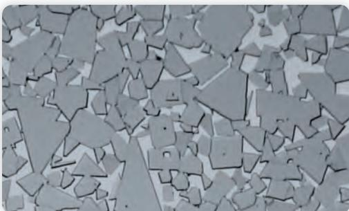
Cross-section through grade B20G tungsten carbide, as used, for example, for hydraulic milling cutter tools
